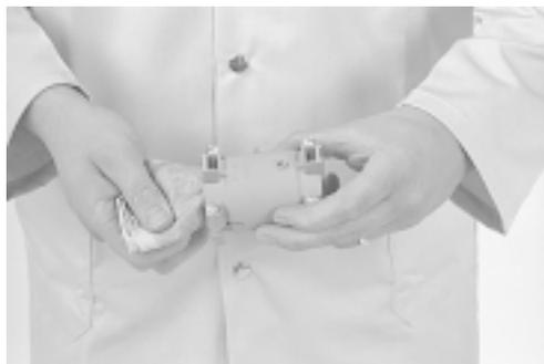
Place the cleaned fitting carefully on the working surface. Avoid any moisture or dirt getting inside the fitting.
