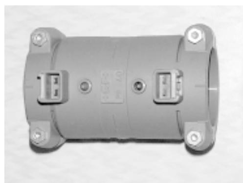
All the pipes have a line down one side and the fittings have external marks every 45° these enable installers to keep prefabricated pipes and fittings in the correct alignment when doing electrofusion joints on site.
