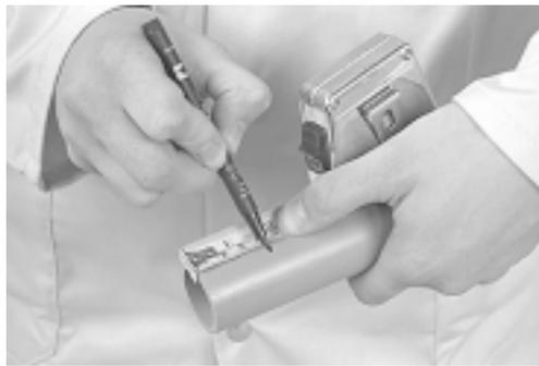
...or mark insertion depth from centre mark on fitting
