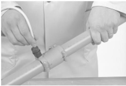
To make an electrofusion joint simply plug the welding cable from the electrofusion control unit, into the electrofusion fitting.
