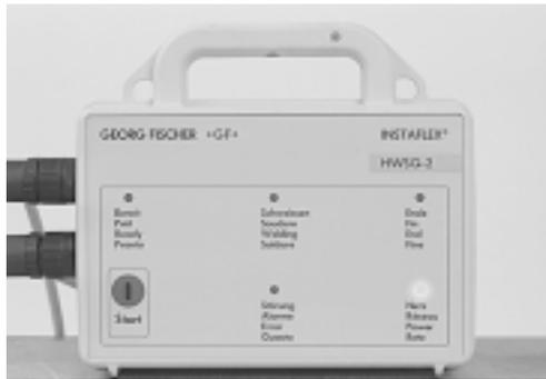
If the alarm light comes on, there may be a fault with the unit and George Fischer Sales Ltd. should be contacted Tel: 01203 535535.
