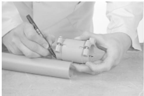
Mark the insertion depth on the pipe after it has been cleaned.
