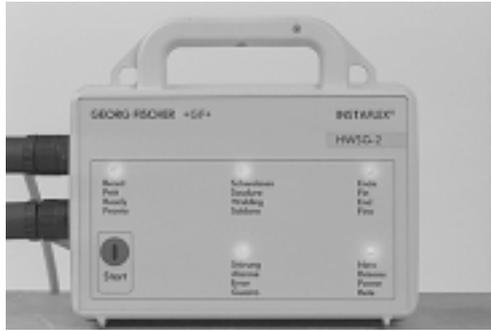
Plug the control unit primary cable into a power source. All the lights on the front of the control panel should illuminate briefly while the control unit conducts a self diagnostic test.
