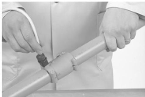
As the electrofusion control unit is fusing the pipe and fitting together, a little indicator pip will rise from within the fitting to indicate a joint has been successfully made.
