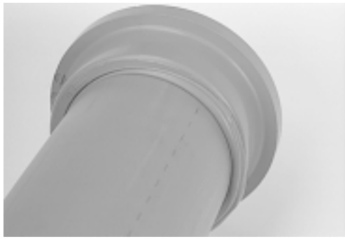
Misaligned bench mounted fusion joint
