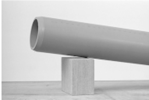
Keep the clean pipe end off the surface
