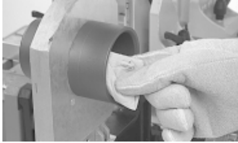
Clean inside the socket
