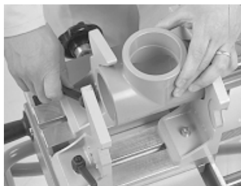
Adjust rear clamps to grip fitting
