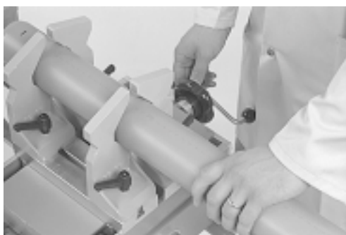
Hold the pipe in the clamps
