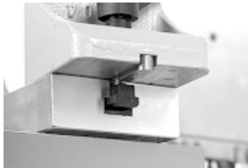
Slide the clamps onto the rail
