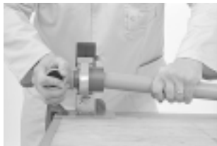
Misaligned bench mounted fusion joint
