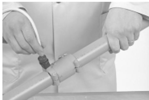
Remove the welding cable
