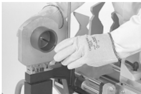
Tighten the bolt with an allen key to secure the bushes in place
