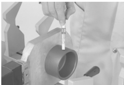
Check heater is switched on
