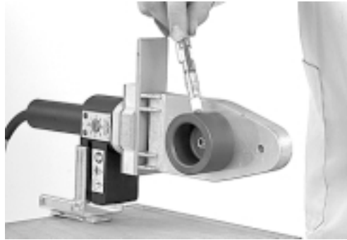
Yellow temple stick is used to check the element has reached the correct temperature _It should melt
