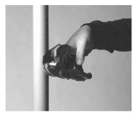
**4.** Wait after the cooling time befor cutting the part in excess.
