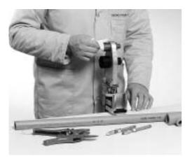
**7.1.3 Cut the pipe** Cut the pipe at right angle, if necessary remove swarf from inside.
