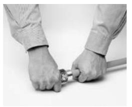
**7.1.4 Chamfer the PP-R/ALU/PP-R** In case of PP-R ALU pipe to take off the aluminium film use the suitable tools.
