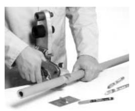
N.B. Cut the pipe ends of 5 cm.
