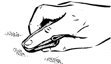
Polish corrosion marks to prevent further damage.
